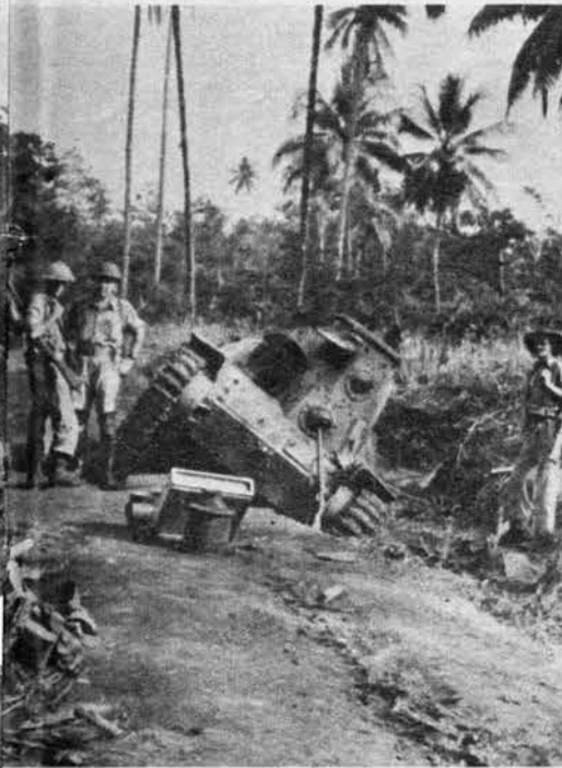
The 2597 is first of series to mount 37-mm. cannon in turret. Its large rear idler provides greater ground traction. The later models may have heavier armor plate, wider track, and an intercommunication system.
